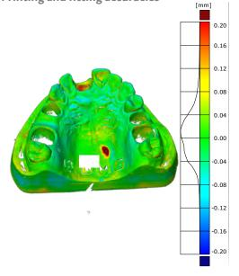
Superimposing the STL file and the scanned printed model indicates the validated accuracy
