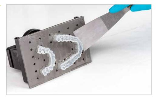
In the case of highly adhesive objects, carefully hit the handle of the spatula with a hammer to detach the baseplate of the printed object from the building plate. Always be careful not to damage the splints.
