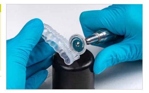
Rotating instruments for manual post-processing
