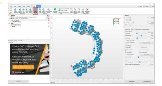
Adding new support bars in Autodesk Netfabb using »create new bar« (red marking) After completing the manual support set-up, check the splint again for correct positioning of the bars and make sure that all bracket pockets are supported. Click on »Apply« to apply the current supports and return to the building plate view.
