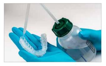
Removing liquid resin residues using isopropyl alcohol
