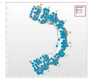
To set new bars, select the function »Create new bar« in the upper menu toolbar. Double-click on the point on the splint to be supported to create a new support bar (alternatively: left-click to set an anchor point, right-click on the anchor point and click on »Create bar«).
